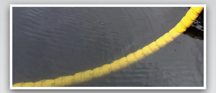
Each cable, umbilical or flexible has a minimum bending radius, below which the cable can be severely damaged and become unusable for operation. If no prevention is taken, overbending will usually happen. In subsea applications this is usually either at the platform or at the seabed.
